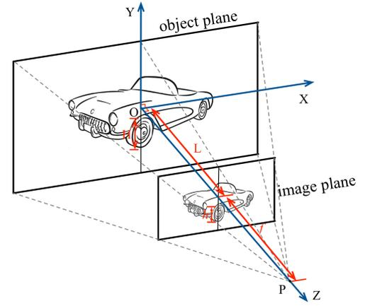
(a) The pin-hole model of the camera system.
