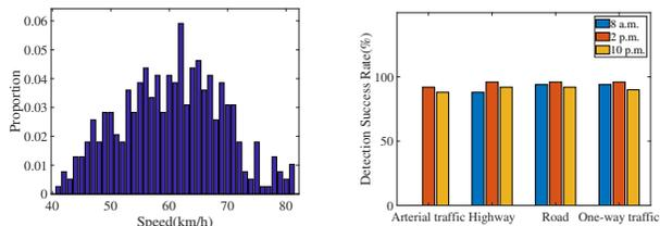
(b) Speed distribution of multiple automobile. (c) Detection success rate in different locations at different time.
