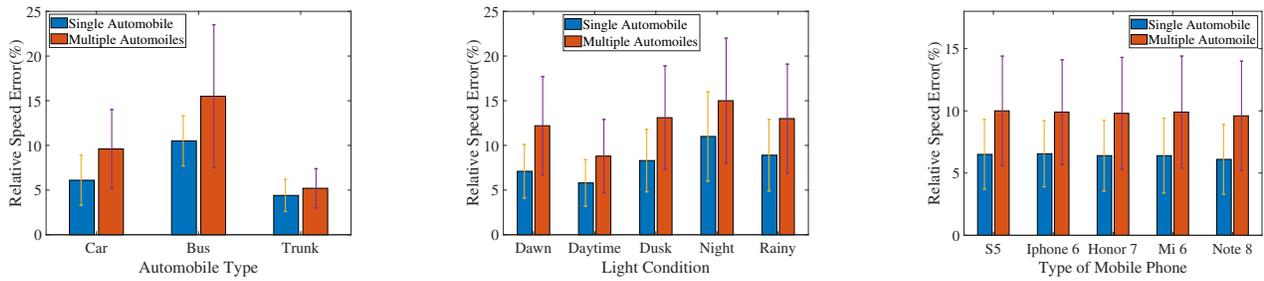
(a) Average relative speed error VS types of automobiles. (b) Average relative speed error VS light condition. (c) Average relative speed error VS type of mobile phone.
