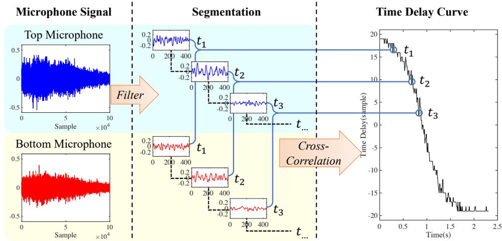
Fig. 15: Illustration of generating time delay curve.
